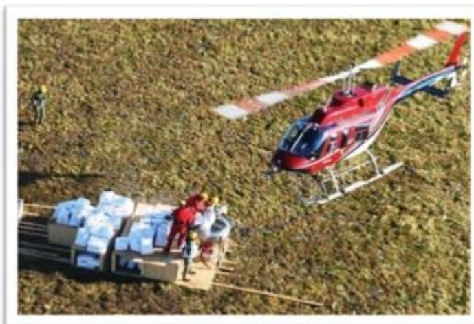
Figure 14. Bait loading platform for refilling of spreader bucket.
