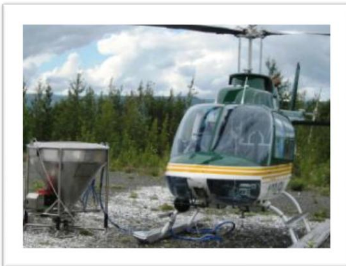
Figure 10. Helicopter spreader buckets used for aerial broadcast of bait pellets.
